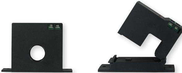
The **Series CCT40/50 Current Transformers** are a low cost alternative for measuring power and monitoring the operation of fans, pumps, or other equipment. For use on existing installations, split core models can be installed without disconnecting cables. Each model offers three jumper selectable ranges and a choice of three different outputs.
